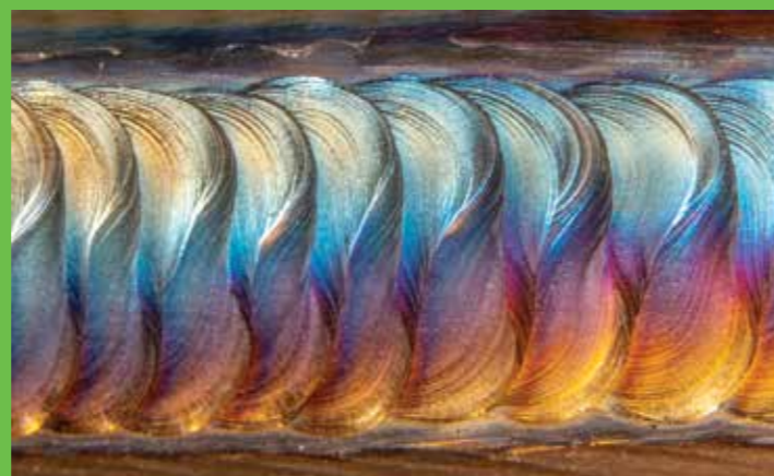
Good regular cap profile by the use of the 'walking the cup' technique.
